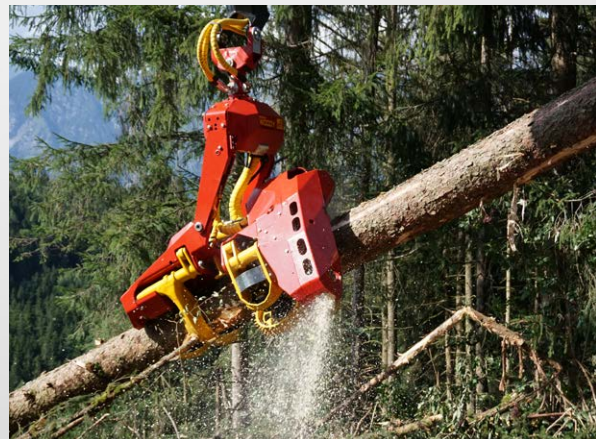
The WOODY has a long overall length, which enables the controlled felling of strong trees.
