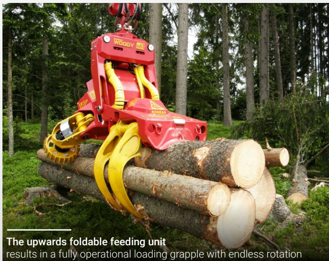
The WOODY has a long overall length, which enables the controlled felling of strong trees.
